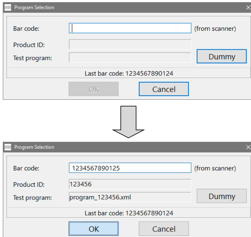
Fig. 68+69: Barcode dialog at the test start
