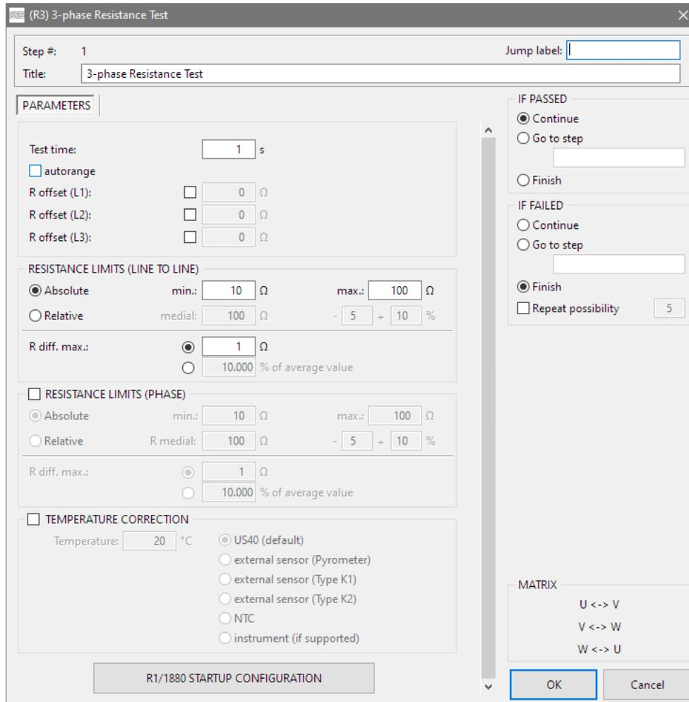
Fig. 46: Test parameters "3-phase resistance test" (R3)
