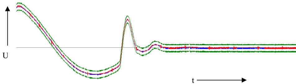
Fig. 82: Tolerance band method
