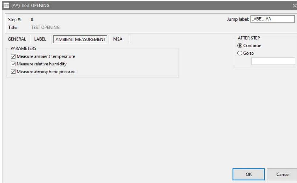
Fig. 40: Tab "Ambient measurement"
