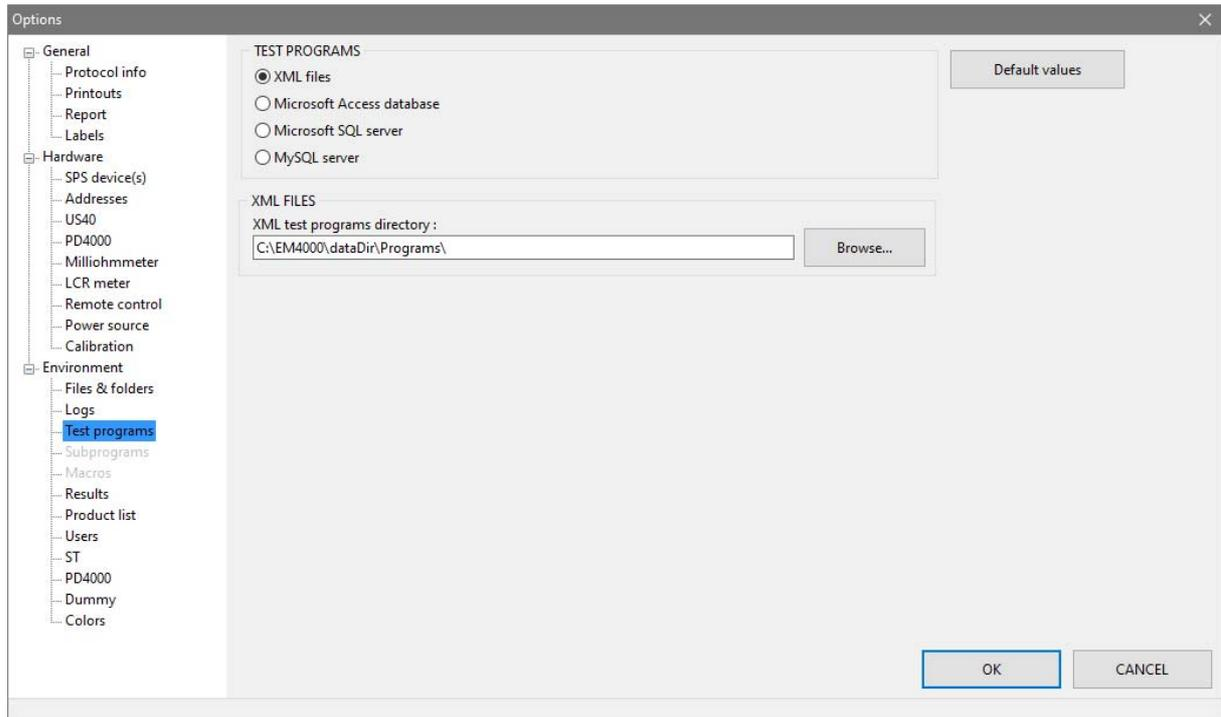
Fig. 21: Tab "Test programs"
