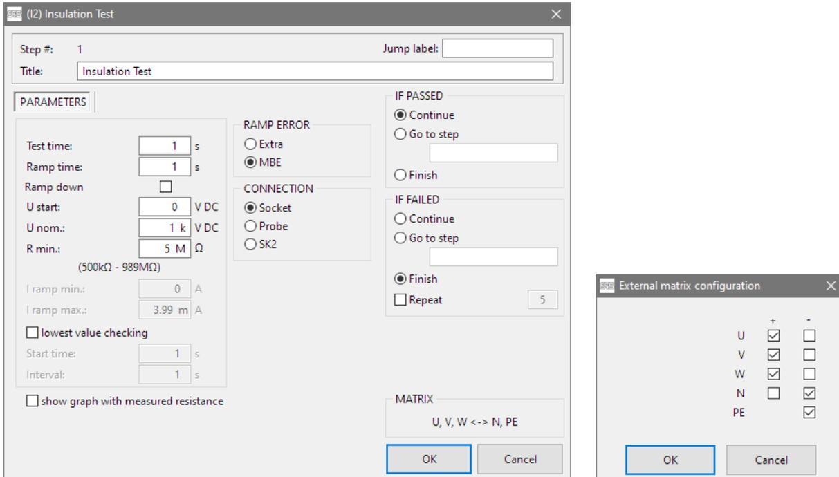
Fig. 47 + 48: Test parameters "Insulation Test" (I2)
