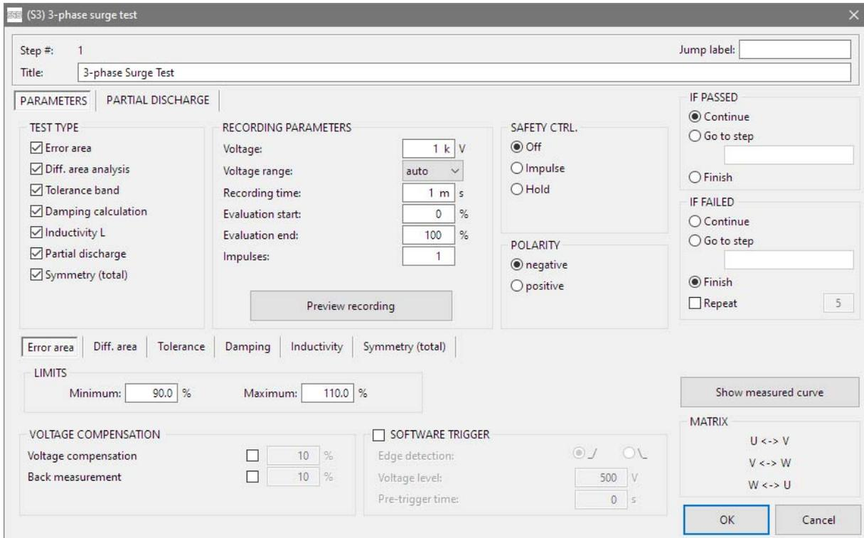
Fig. 58: Test parameters "3-phase surge test" (S3)
