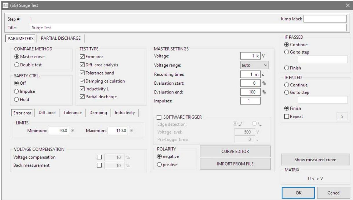
Fig. 83: Test parameters of surge test
