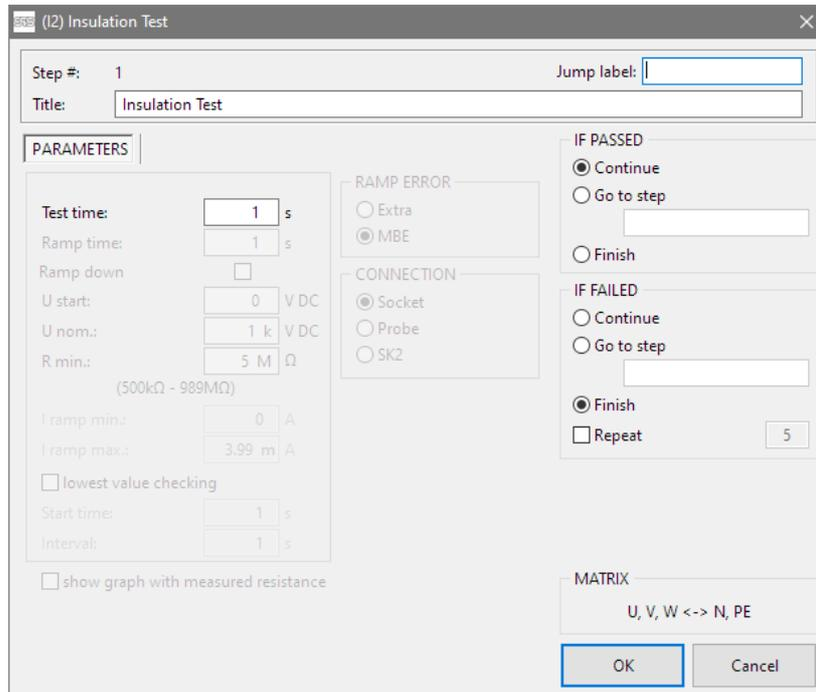
Fig. 37: Dialog window with test parameters (example)
