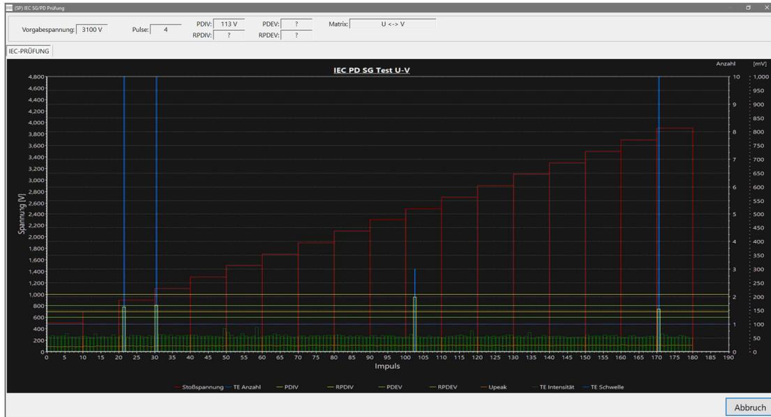
Fig. 75: Display during "IEC PD-SP Test"
