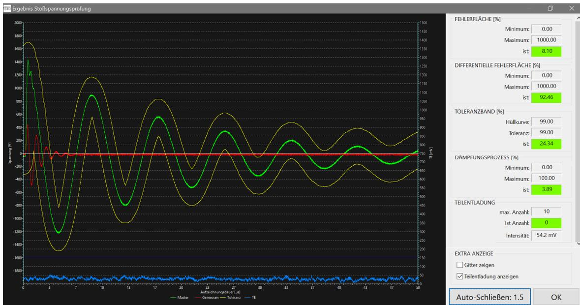
Fig. 74: Window "Result of surge test"
