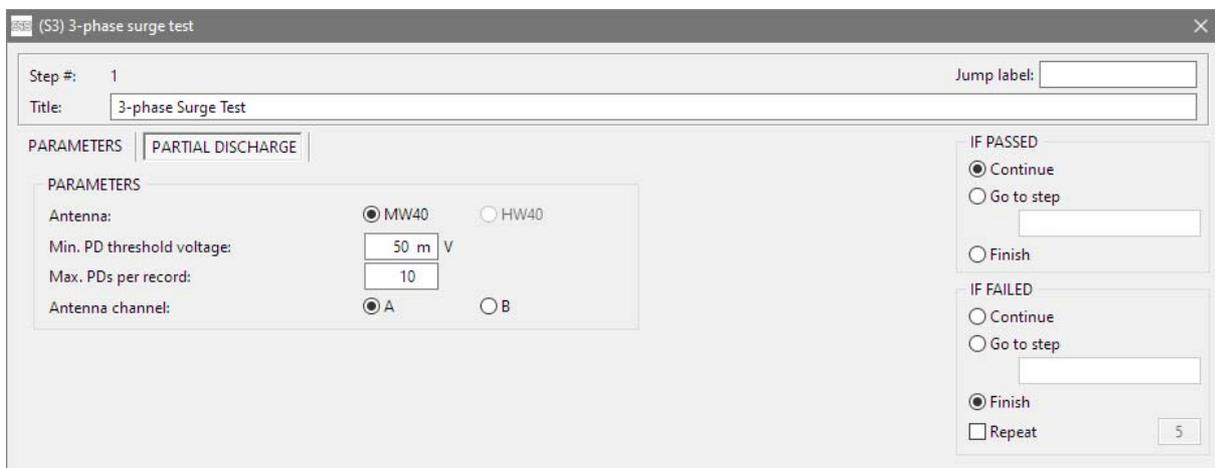
Fig. 59: Test parameters for partial discharge evaluation)
