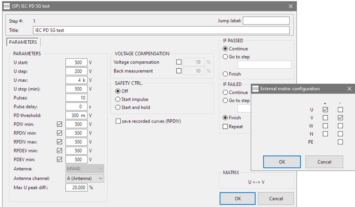
Fig. 60+61: Test parameters "IEC PD surge test" (SP)
