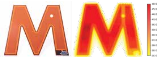
SmartHeat SLT heater intentionally damaged by a hole punch (left, visual image). Heater is shown to continue operating in areas surrounding the damage (right, thermal image).
