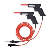
Elabo safety test probes with high-voltage cable and special high-voltage plug connectors. The test probes are authorised for a voltage of 8 kV AC/10 kV DC. Consequently, we have provided other connector sockets on the test devices with a higher output voltage. All test probes can also be obtained as single items.
