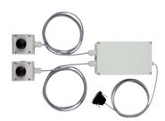
According to EN50191, use of a two-hand control according to EN 574 type IIIC and EN 354-1 at the test bench is indispensable when using fixed connected test conductors. The safety two-hand relay consists of an analysis unit and two separate pushbuttons. The unit can be directly connected to Elabo high-voltage test devices.
