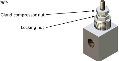
If a leakage is detected when the valve is closed, the following procedure has to be followed:
