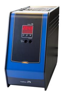
The Traqc-3 LL dry block calibrator is a high precision Laboratory temperature calibrator ranging from -30°C up to 150°C. This instrument is equipped with a special patented heat / cooling section which creates a superb axial homogeneity. This ensures an accurate and stable temperature calibration.
