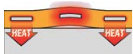
Voids or bubbles beneath the heater cause localized hot spots which can result in premature heater failure
