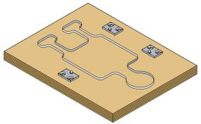
**Stiffener**: Flexible or rigid pieces of material (usually polyimide or FR-4) added to flex circuits to reinforce them for component mounting. There are no conductors on stiffeners, as compared to rigid-flex circuits.
