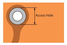
**Annular ring**: The minimum width of the exposed copper or solder that surrounds a flex circuit's through-holes.
