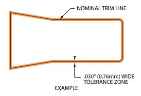
profile tolerance zone. The circuit trim line could vary anywhere inside the zone.
