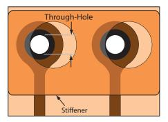
or cover access hole is flush with the edge of a through-hole.
