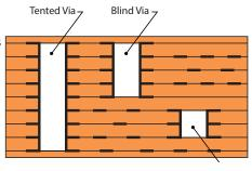
the top or bottom conductor layer to adjoining layers, but the via does not extend through all layers. A buried via only connects internal layers and is not exposed in the finished circuit. Blind and buried vias increase circuit cost, but they free up space for additional conductors on the non-drilled layers.
