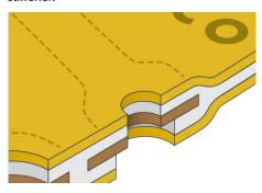
**Nesting**: Designing circuits so that they lay closely together on a panel during production. This maximizes the usage of panel space, which minimizes production cost.
