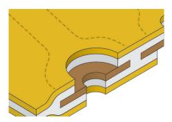
**Minor access hole**: An access hole (see "Access hole") that exposes only a very small portion of a conductor pad, used on holes where a solder pad is not needed or desired. The cover hole must still be larger than the through-hole to allow for normal registration tolerances. Generally against a component or a stiffener.
