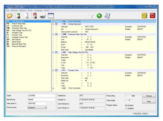
In editor mode intuitively different test programmes can be created which can be adapted flexibly in regard to the desired test methods and the cycle time:
