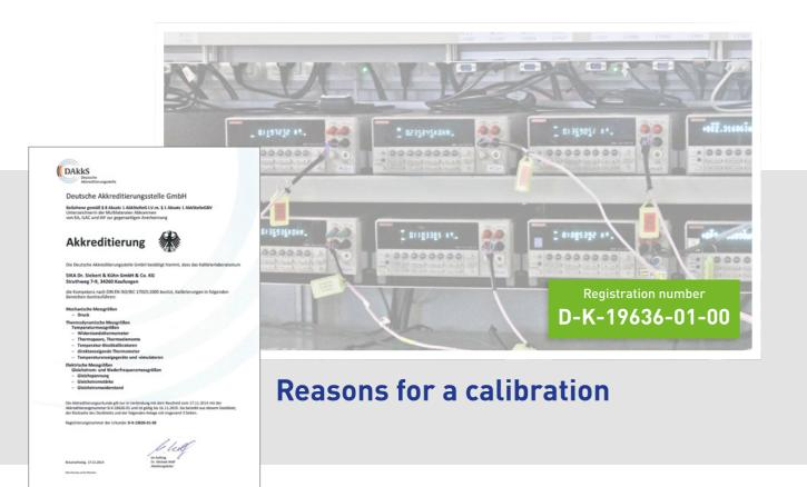
Temperature sensors are subject to mechanical, thermal and chemical stress. This results in a drift the longer the sensors are in use. Only the regular calibration of the sensors provides information on the difference between the actual temperature and the measured temperature and makes the specific drift visible.
