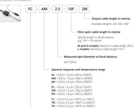
FC = FibreCube fibre optic infrared temperature sensor
