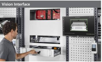
The Vision Interface enables you to automatically inspect components. In this way, faulty wiring or assembly of components can be detected using camera technology and the passing on of an incorrectly assembled product can be avoided.
