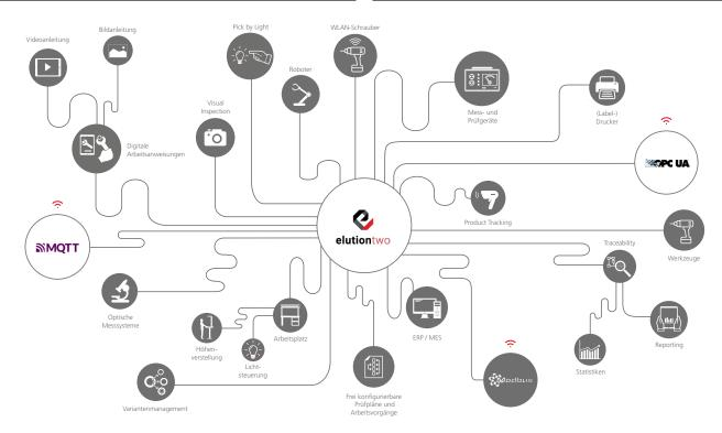
The MQTT interface is an open message protocol which has become the standard protocol for IOT or machine-to-machine communication between devices and applications. In the future, MQTT-capable devices will be able to communicate directly with the elution two.
