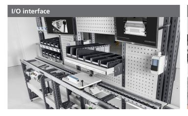
The I/O interface makes it possible to independently integrate digital inputs and outputs into the process. These can be sensors and actuators that monitor and control your process or supply it with additional information. For example, environmental conditions such as temperature or humidity could be recorded.
