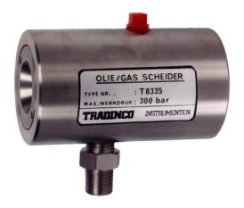
The oil/gas separator model 8335 is used for oil-free testing and calibration of pneumatic instruments when using a hydraulic pressure source, such as a hydraulic deadweight tester. Tis separator has no diaphragm between the two media and therefore does not affect the accuracy of measurement. The level of separation can be checked through the monitoring glasses.
