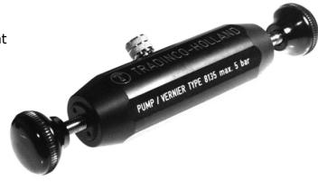
Our hand pump/volume regulator 8135 is a very handy tool for the generation and adjustment of pneumatic pressures. This unit can generate pressures up to approx. 5 bar. The plastic casing of the pump is designed to assure maximum grip. This material also prevents heat transfer by e.g., hand warmth.
