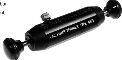
Vacuum hand pump/volume regulator 8125 is a very handy tool for the generation and the adjustment of vacuum pressures. This unit can generate vacuum pressures down to approx. -0,75 bar. The pump's plastic casing is designed to assure a maximum grip capability and the material prevents heat transfer by e.g., hand warmth. The pump is compact, lightweight and rugged, making it ideal for field use. The simple design and quality construction ensure a long service life.
