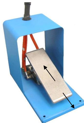
Dual function foot control valve. Pressing forward activates clamp installation. Heel action activates tail return and prepares for next clamp.
