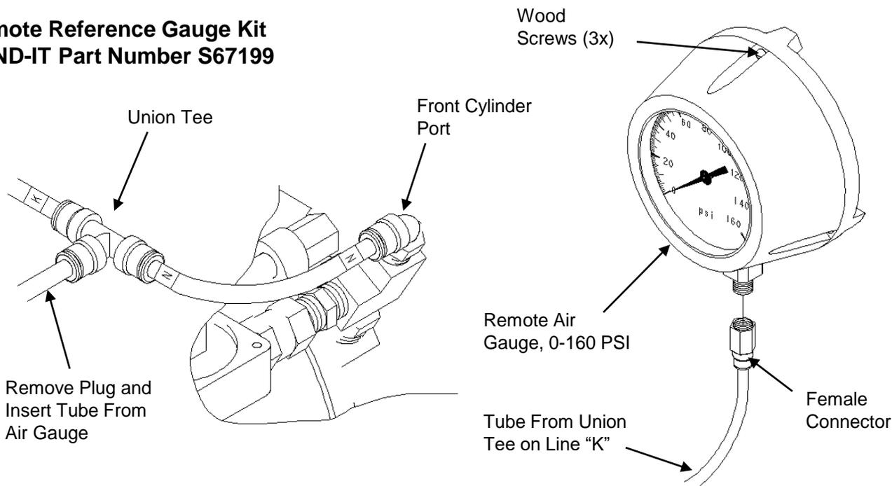
The Remote Reference Air Gauge will read air pressure in the front of the cylinder for both pull-up and holding pressures. To read gauge: When tensioning a clamp, the maximum pressure the gauge reads during the cycle is the pull-up pressure. After the tool switches over to the lower pressure holding cycle and before the clamp is rolled up in preparation for lock, the pressure shown is the holding pressure.
