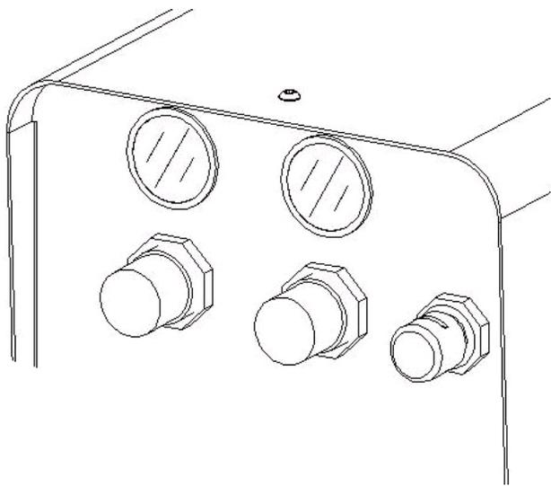
Air pressure setting can be made using the regulators and gauges on face of the tool.
