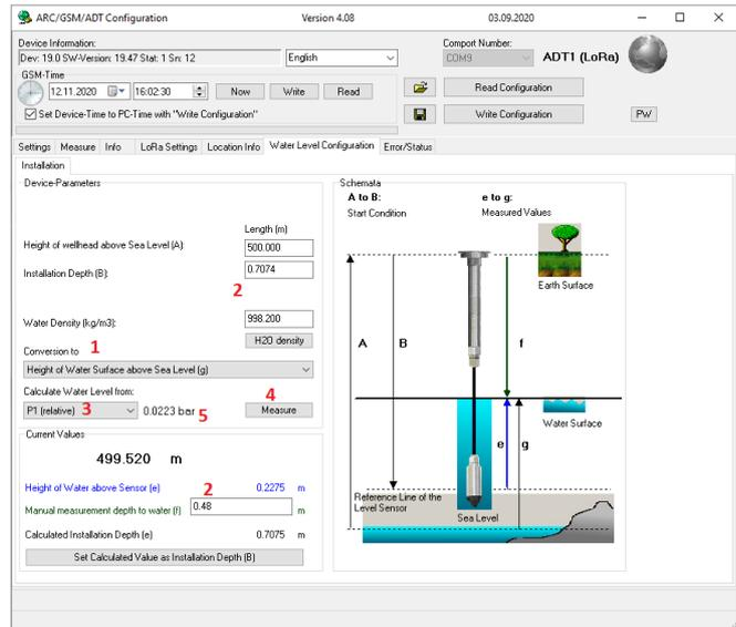
Thus, the height of the water column **e** above the sensor is 0.7075 m. To this value must now be added the length of the inner part of the ADT1 housing, 16.5 cm.
