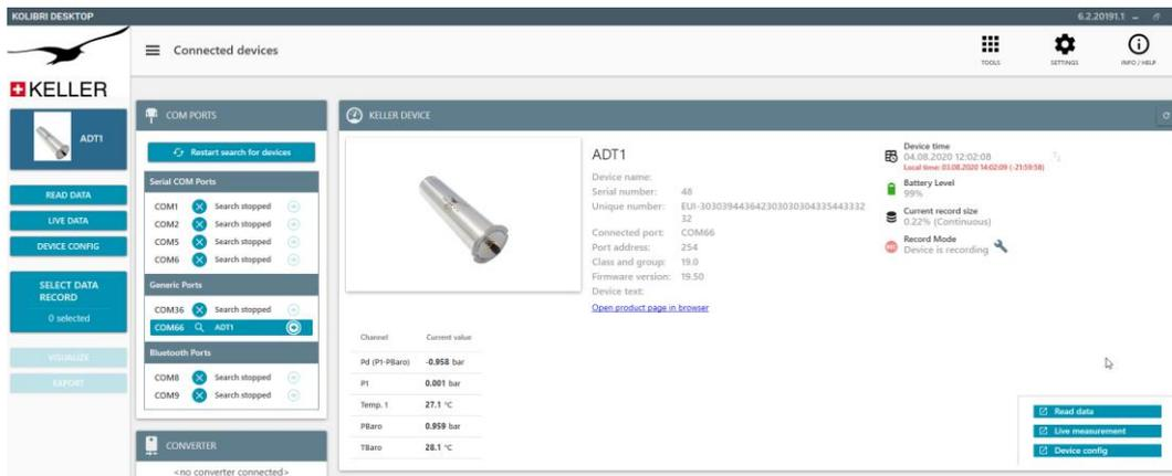
The connection to ADT1 is now established automatically and all available RECORDs appear. Select the desired RECORD and click on the button "Start reading selected record from device".
