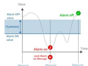
**NOTE:** If the alarm condition is active and X alarm messages are sent no more alarm message will be sent. The alarm is only re-armed when the Alarm OFF condition is fulfilled.
