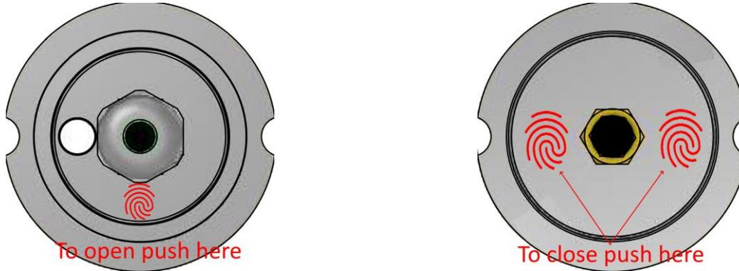
To close the unit, push with two fingers against the top of the housing/piston until it stops. Be sure that that the piston is completely inserted. Keep dry before opening and closing. To close the ADT1 Box you just squeeze the screws together and make a quarter turn.
