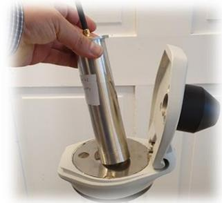
Measure and note the distance  $B$  from measuring point to water surface.
