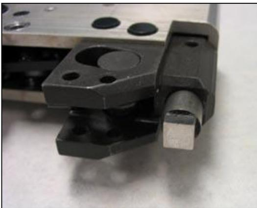
Once the pin is removed, grasp the Knife Assembly with a pair of needle-nose pliers and pull out of tool head. Examine for wear and rotate or replace if needed.
