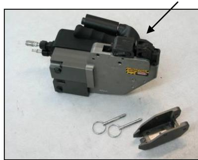
2. Remove Flip Cover and Tension Block Assembly for cleaning and lubrication.
