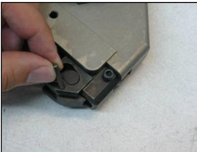
3. Remove the Cutter Blade Pin and Cutter Blade.
