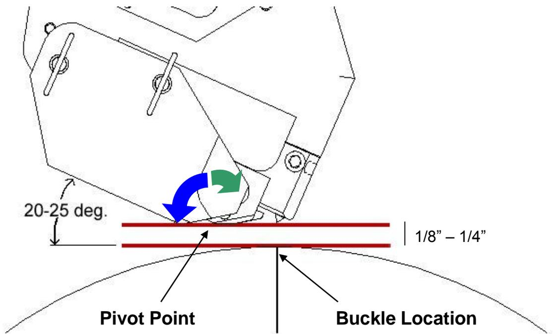
As the band is tensioning, the tool may rotate clockwise up to 5 degrees about the pivot point (Green Arrow). During the cut-off cycle, the tool must be allowed to rotate counter-clockwise up to 35 degrees (Blue Arrow). Because of this movement, **BAND-IT recommends that the tool be mounted in a fixture that will provide adequate rotation during both cycles.**
