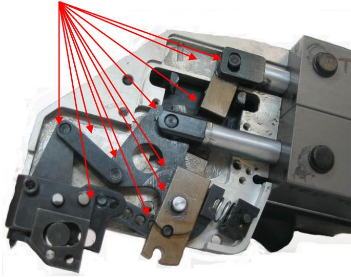
After the Maintenance Flip Cover is cleaned, lubricated, installed and Quick Release Pins are in place, apply tension to the Flip Cover Screw and Head Screws. Refer to **pages 7, 17.**
