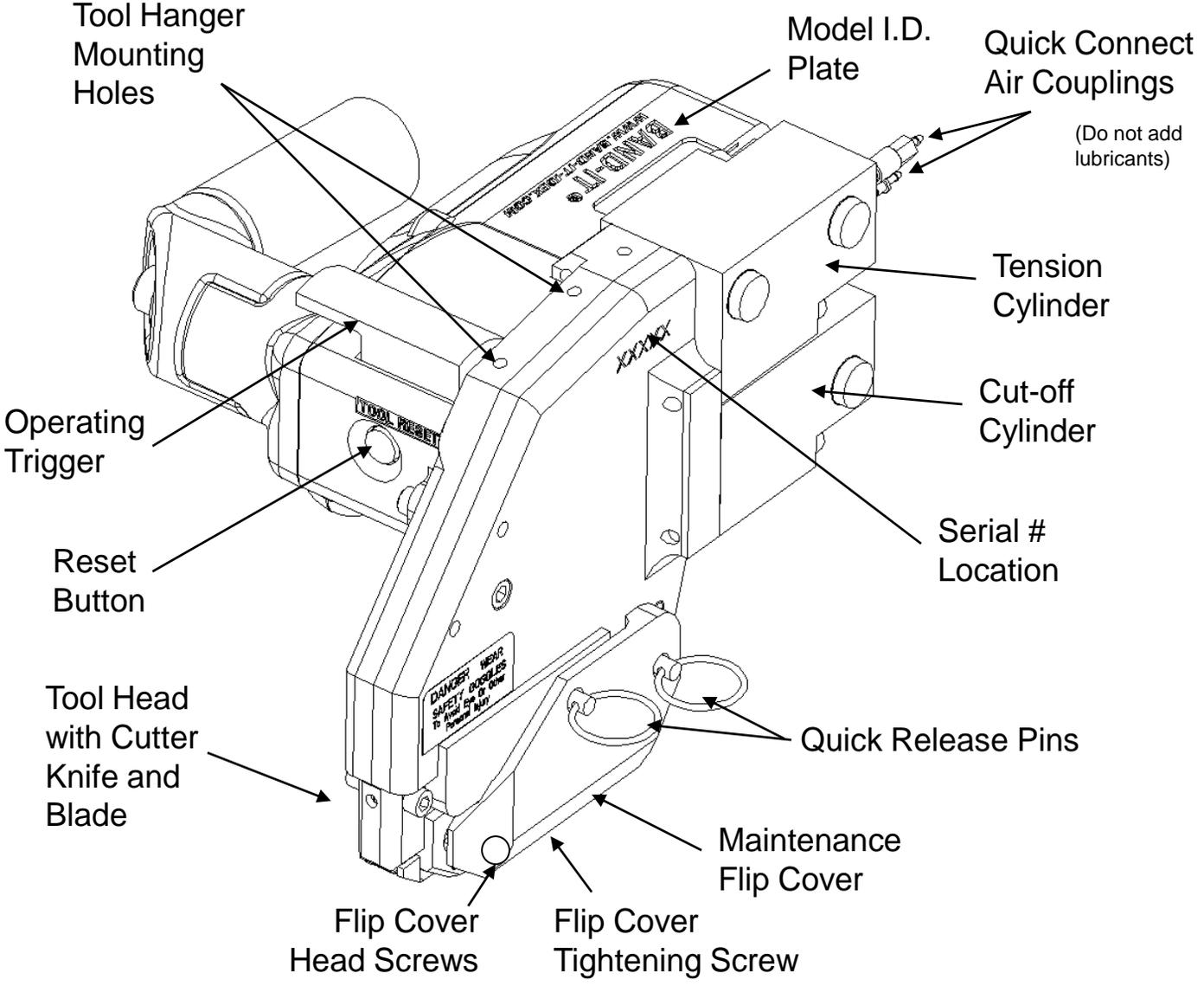
**Important:** Before disassembling tool, be sure to shut-off air supply on the Air Controller Module.
