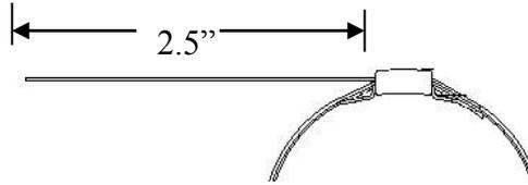
1. Insert clamp tail into tool as shown. Clamp tail length extending into tool must be at least 2.5" (6.4 cm) long. The head of the tool should rest against the buckle. **Note - Do not activate tool while inserting clamp tail. This can cause clamp tail to jam in the Tension Block Assembly.**
