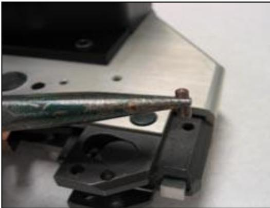
To remove Cutter Knife Pin the Knife Assembly must be in its uppermost position indicated by the Cutter Knife Pin in line with the access hole. If not aligned, connect the tool to the Air Controller Module. Open the Air Shut-off Valve to momentarily pressurize the tool. Close the valve and disconnect the tool from the Air Controller Module. Then push out the Cutter Knife Pin with a piece of wire (for example, a bent paper clip).
