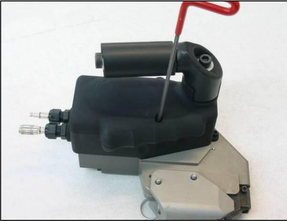
The Timing Valve will be affected over time by contaminants in the air system. Moisture, dirt particles, oil and solvents can cause blockage or fluctuations in the tool performance.
