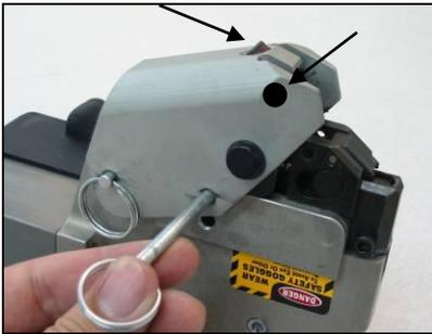
1. Loosen the Flip Cover Tightening Screw and Head Screws (**see note above**) to remove both Quick Release Pins as shown.
