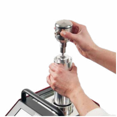
Dry block calibration Aseptic sensor
