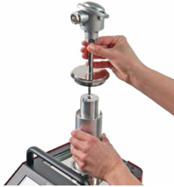
Dry block calibration Flange sensor
