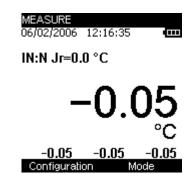
The **Measurement** mode makes it possible to display the Min (bottom left), Average (bottom centre) and Max values (bottom right) from the last **RAZ Min/Max** command.
