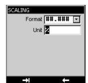
Once the parameters have been set, the scaling is automatically enabled. To disable it, enter the **Configuration/Scaling** menu, select **OFF** and confirm by pressing the **VAL** key.
