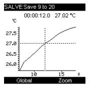
At this level, you can display the whole curve or a zoom around the cursor. The cursor is moved using the navigation keys( $\leftarrow$  and  $\rightarrow$ )
