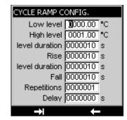
Use the F2 key to access the CONFIGURATION/RAMP menu. Attention: the appropriate function mode must be programmed (Single Ramp mode) to access the CONFIGURATION/RAMP/CYCLIC RAMP menu.
