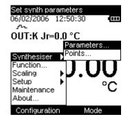
Once you have selected the configuration/Synthétiseur/ Paramètres (configuration/Synthesiser/Parameters) menu, confirm by pressing the VAL key.
