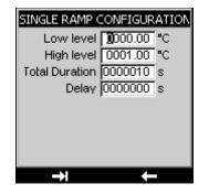
Use the **F2** key to access the **CONFIGURATION/RAMP** menu. Attention: the appropriate function mode must be programmed (**INCREASES** mode) to access the **CONFIGURATION/RAMP/SINGLE** menu.
