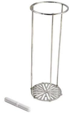
The magnetic stirrer ensures a uniform temperature distribution in the calibration liquid.
