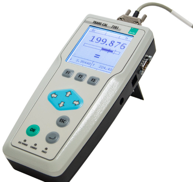
Diagram 6: TRANS CAL model 7281 Sub-D female connector (measurement, sensor test, voltage source)
