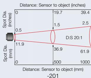
Sensors can measure at longer distances than shown, with a larger measured spot size. Diagrams show the diameter of the measured target spot versus the distance from the sensing head (90% energy).
