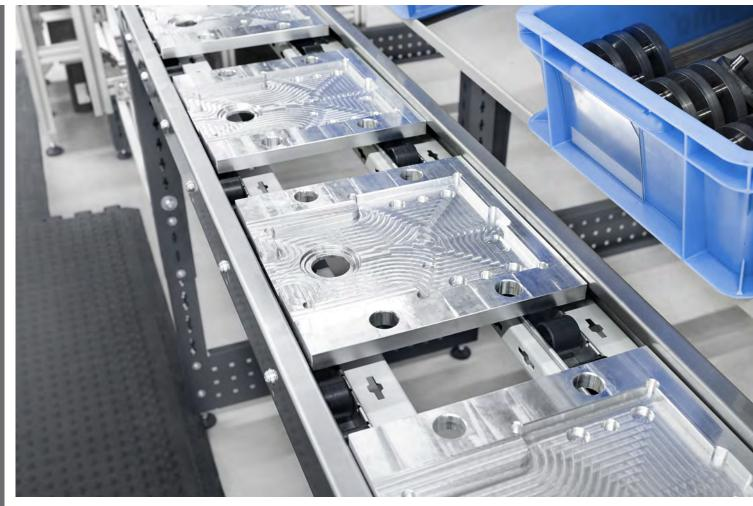
Guarantee smooth and efficient material flow with avero handling lines. The workpiece carrier rolls gently over the roller tracks of the avero workstation system from assembly segment to assembly segment.
