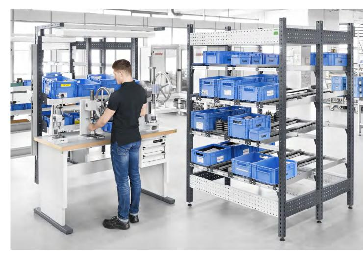
Make sure of optimum and efficient material provision in your manual assembly – with avero FIFO shelves! You remove the parts at the front of the assembly workstation, while the necessary supplies are continually provided from the back.
