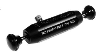
Vacuum hand pump/volume regulator 8125 is a very handy tool for the generation and the adjustment of vacuum pressures. This unit can generate vacuum pressures down to approx. – 0,75 bar. The pump's plastic casing is designed to assure a maximum grip capability and the material prevents heat transfer by e.g. hand warmth. The pump is compact, lightweight and rugged, making it ideal for field use. The simple design and quality construction ensure a long service life.
