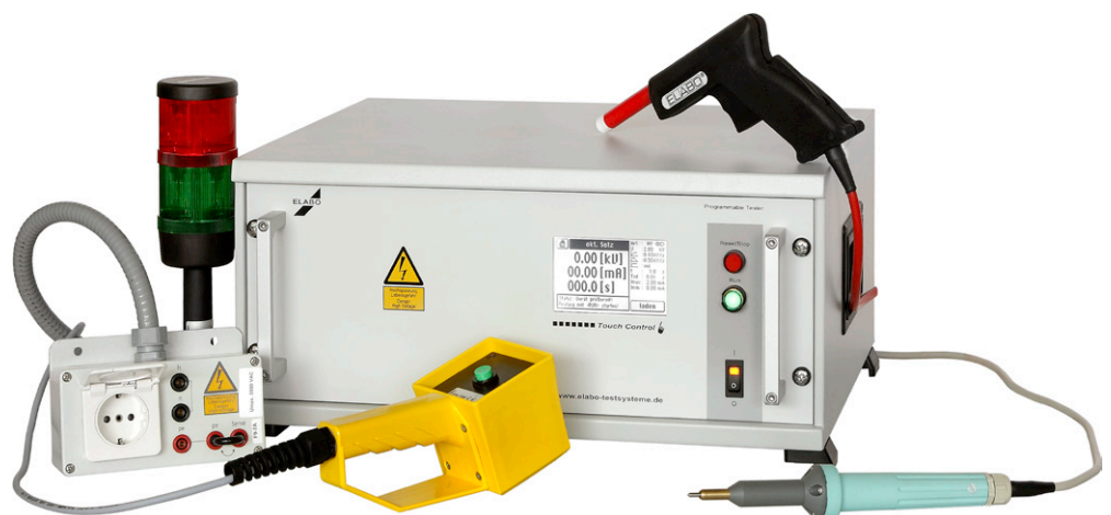
Fig. 3.1: Tester with display and accessories installed in 19" / 4HU housing
