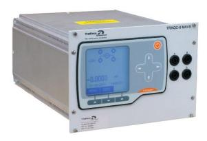
The Traqc-9 MAVS allows you to power your transmitters and measure the common mA or V output signals precisely. In addition to this, this instrument offers you the required functionality for loop testing. An intelligent switch test function completes it all. You only need to connect the Traqc-9 MAVS once and you're ready to calibrate your transmitter and loop in a fast and easy way.
