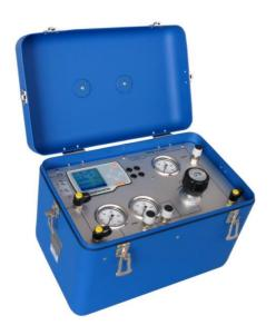
The digital pneumatic portable calibrator Traqc-8 is designed for the supply and measurement of high pneumatic pressures. The Traqc-8 can be used for calibrating and testing high pressure transmitters, pressure switches, safety valves, etc. The built-in high pressure gas bottle and battery make it possible to use this test unit at all locations, independent of any external pressure source or mains supply.
