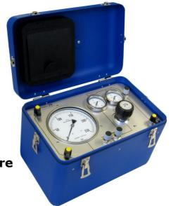
The analog pneumatic portable calibrator Model 8185 is designed for the supply and measurement of high pneumatic pressures. Model 8185 can be used for calibrating and testing high pressure transmitters, pressure switches, safety valves, etc. The built-in high pressure gas storage system makes it possible to use this test-unit at all locations, independent of any external pressure source.
