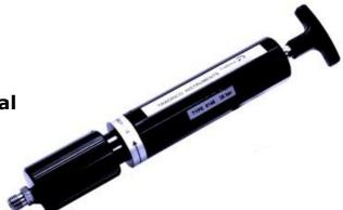
This calibration Hand Pump/Volume regulator" EASYPRES" makes generating pressures up to 25 bar easier than ever before. This double action pump system generates test pressures with a minimum number of strokes and requires minimum effort to reach high pressure.
