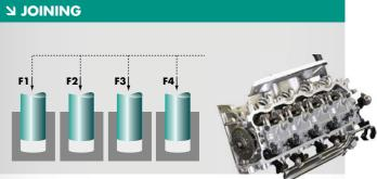
Multichannel monitoring of joining process in cylinder head assembly. The synchronous process during the assembly of valve seating rings and valve guides is measured and analyzed. DigiControl PC software logs and visualizes the process data from up to 32 controllers.
