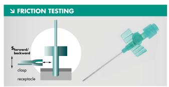
Testing the ease of movement of a venous canula over the length of the steel insertion needle. The clasp holds the canula and moves it up and back over the needle.
