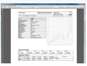
A Data-log wizard provides filters for selecting and displaying stored measurement logs. A report printout containing component data, curve information and all evaluation results can be generated for each individual measurement log.
