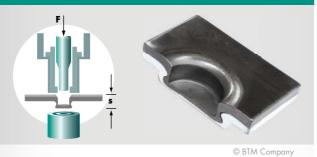
The flow process produced in the two sheet metal parts by the clinching stamp and die is monitored by a force/displacement measurement.
