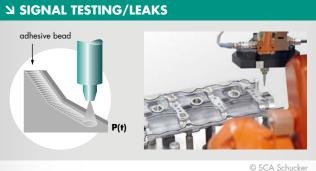
Checking for continuous application of adhesive beads, e.g. to prevent leaks from gaps in the adhesive joint. This is done by monitoring the pressure/time curve in the dispensing line.
