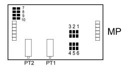
PT1 - Fine Gain Adjustment. (Additional P2 potentiometer on input module ME).
